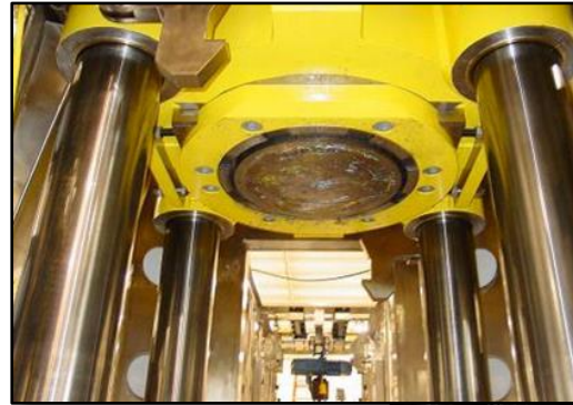
The Supercompactor used to treat transuranic waste at AMWTP
